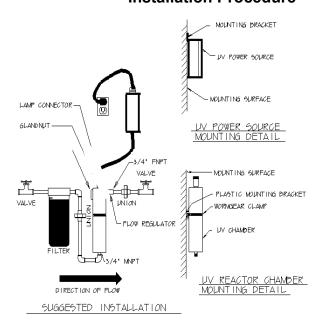
The UV disinfection system should be the last step of your water treatment system. Choose a location for installation with a close electrical outlet. Note the direction of water flow in the supply line.
